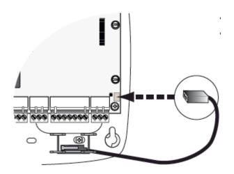
• Wiring an off-the-wall tamper:
